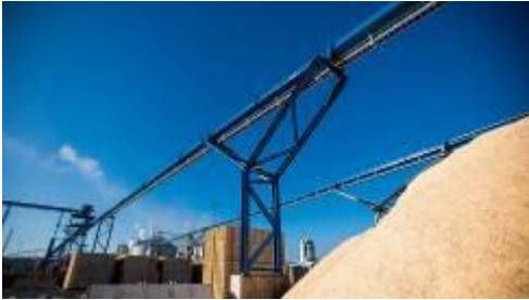
Photo 1: In the wood and biomass sector, Vecoplan has delivered and commissioned many machines and systems in recent years – such as these transport systems for sawdust and wood chips.
