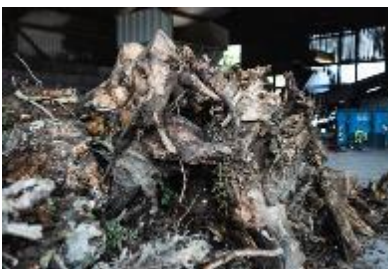
Photo 2: Waste wood and root wood mixed with minerals are easily pre-shredded during the ripping procedure, ready for subsequent processes
